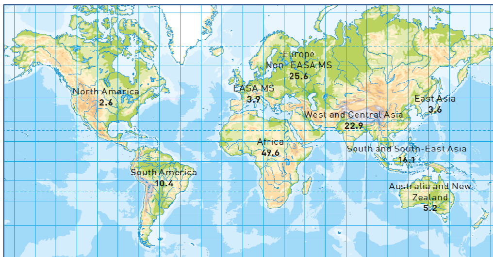
Figure 10 Rate of fatal accidents per 10 million flights per world region (2000–2007), scheduled passenger and cargo operations) (Source: EASA)
